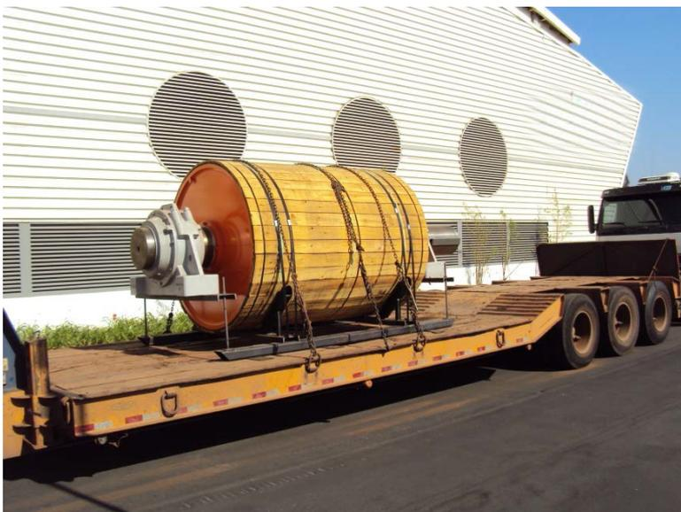
Figure 9 – Standard Pulley Packing
